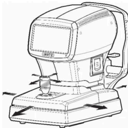
[Operating the joystick for left/right & focus adjustment]
